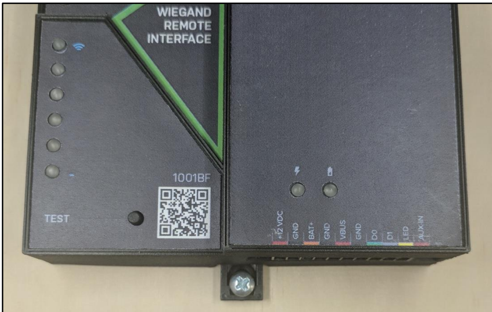
Figure 15: Bottom DIN Rail Screw Mount
